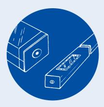
All laser beams must terminate in a beam block that is firmly secured in place. A power meter that can be moved out of the way of the beam is not a beam block; a beam block should be provided beyond the power meter. The beam block must be substantial and suitable for the energy and wavelength involved. It must not produce specular reflections or excessively bright diffusely scattered light.
